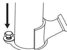
Step 4: Continue to vibrate the rail as illustrated in step 2 and step 3. It can take from 2-4 minutes of vibrating the rail to free the rail from the products of corrosion. The amount of vibrating required depends on the amount of corrosion that has built up in the anchor.
