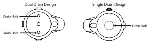
Drain hole configuration will depend on the age or type of the anchor socket.
